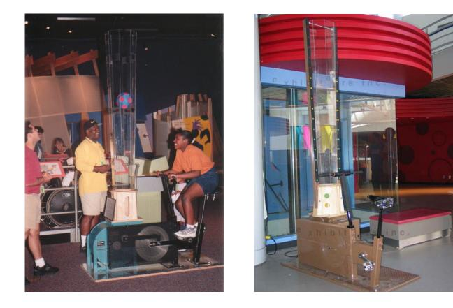
Visitors pedal a bicycle that is connected to a blower. The blower keeps a ball suspended in an air stream. Visitors can measure both their peak energy output (height of ball) and work output (average ball height x time).
