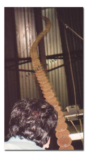
See and feel wave behaviour such as reflection, constructive and destructive inteference and refraction using this unique wave maker that can be up to 60 feet high!
